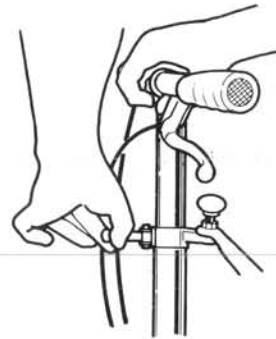
7. Adjust height of the handlebar and secure the handlebar quick release clamp.
