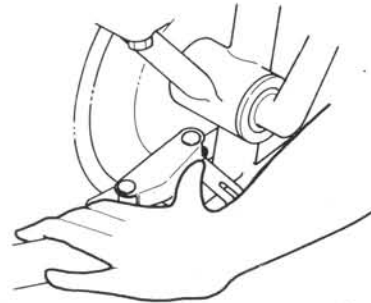
5. Push mid-frame latch horizontally with thumb until locked securely.
